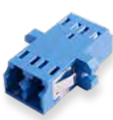
F1-8035 Duplex Singlemode-Blue LC - Style 3 SC Footprint Polymer Housing Zirconia Sleeve
