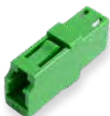
F1-8008 Singlemode - APC - Green LC APC Style 1 Polymer Housing Zirconia Sleeve
