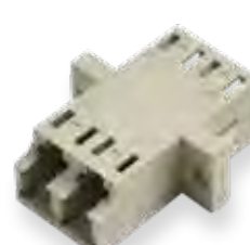
F1-8030 Duplex Multimode-Beige LC Style 3 - SC Footprint Polymer Housing Phos. Bronze Sleeve
