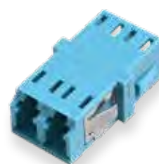
F1-8050NF Duplex Multimode - 10 Gig Aqua (No Flange) LC - Style 5 SC Footprint Polymer Housing Zirconia Sleeve
