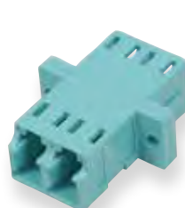
F1-8050 Duplex MM -10 Gig - Aqua LC - Style 3 SC Footprint Polymer Housing Phos. Bronze Sleeve
