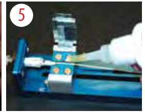
EPOXY FIBER INTO PLACE
