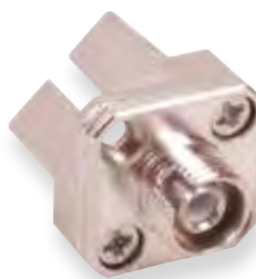
F1-2821CC FC/APC (female) - SC/APC (female) (Square Flange) Metal Housing Zirconia Sleeve
